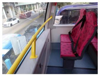
Figure 1- Provision of seat belts at the exposed seats on the upper deck of a FB
