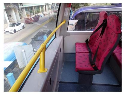
Figure 3 – The horizontal guardrail and the seat belts on exposed seats on the upper deck of a franchised bus
