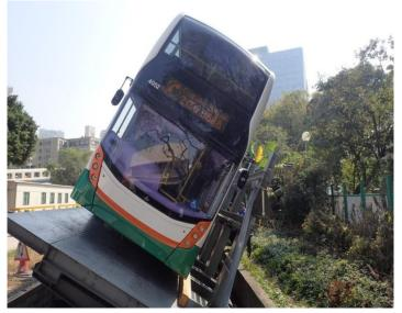
Figure 1 - Stability test to simulate full load condition to ascertain the double-decked bus can be tilted at an angle of 28 degrees
