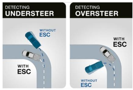
Figure 4 – A picture showing the performance of the ESC
