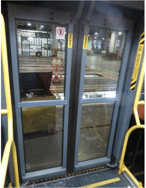
Figure 5 – The additional horizontal guard bar in the middle of the exit door
