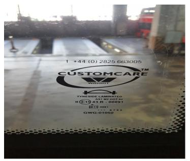
Figure 2 – The marking on the bottom right hand corner of the windscreen at the upper deck of a franchised bus showing the laminated materials applied on the windscreen
