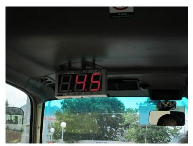
Figure 6 – The speed display unit which is currently installed on a public light bus in Hong Kong
