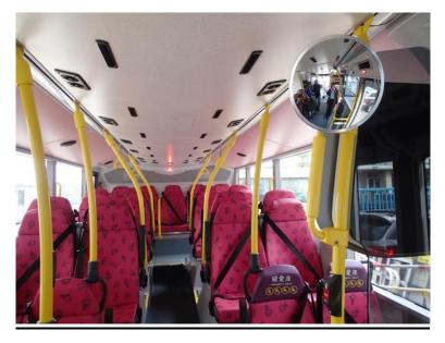
Figure 2 – Provision of seat belts on all passenger seats on the lower deck of a FB
