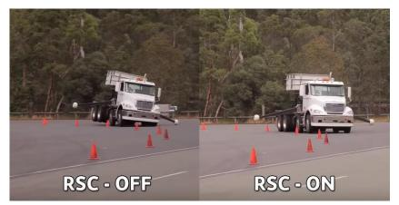
Figure 5 – Demonstration of the performance of a RSC on a truck with high center of gravity
