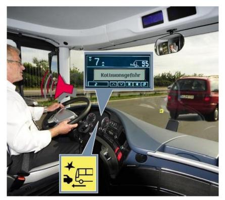
Figure 7 – Demonstration of the activation of the collision prevention system
