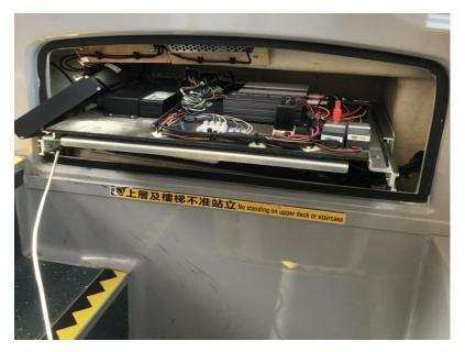
Figure 4 – The black box installed on a franchised bus
