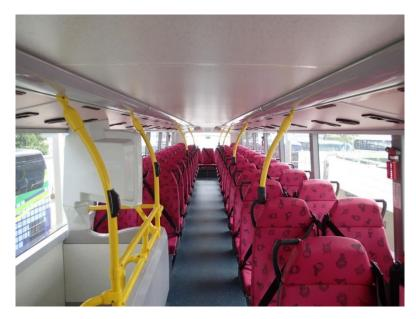
Figure 3 – Provision of seat belts on all passenger seats on the upper deck of a FB
