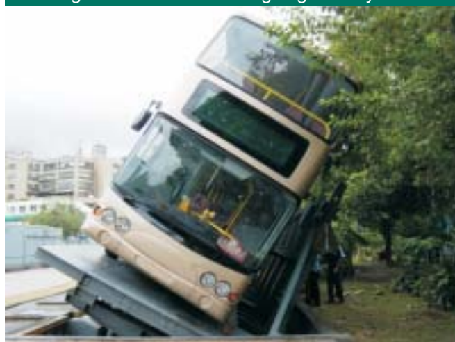
Figure 8.6 – A bus undergoing stability test
