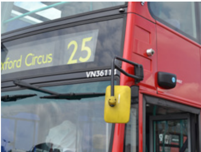
Additional sensors on buses can help to detect cyclists in blind spots.
