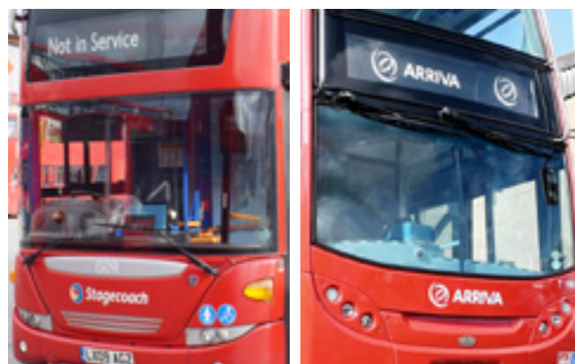
Windscreen wiper protection must be provided, unless they are located at the top of the screen out of harm's way.
