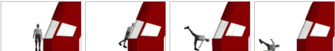
Future buses will have a more sloped windscreen and more rounded corners to help deflect pedestrians more upwards and laterally to reduce run-over risk.
